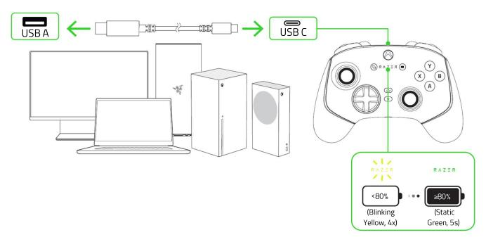
The battery status indicator will appear only when the controller is off, and just once when the applicable power level is reached. Only use the included USB Type A to USB Type C cable to charge the Razer Wolverine V3 Pro. For best results, please fully charge the controller before using it for the first time. A depleted battery will be fully charged in approximately 3 hours.
