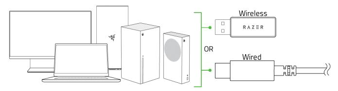
The Razer Wolverine V3 Pro prioritizes wired connection via cable but will automatically switch to the dongle if a wired connection is not detected.
