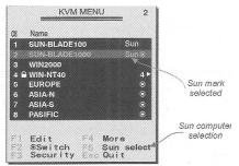
**NOTE:** It is unnecessary to switch the Sun mark ON or OFF if an authentic Sun keyboard is being used on the console. In other words, you must ensure that the Sun-marked port has not been selected if you are already using a Sun keyboard.
