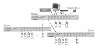
**NOTE:** A device (computer or KVM switch) at any 'PC x' port can be changed at any time after initial power-up. If you change any one of the **PC 1** to **PC 8** port connections from a computer to a Slave KVM switch or vice versa, or replace the devices of a port, the OSD will update this change the next time it is activated.
