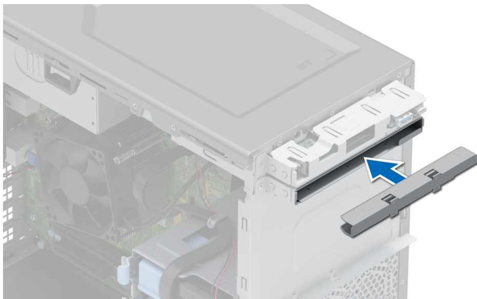
Figure 25. Installing the optical drive filler into the optical drive cage
