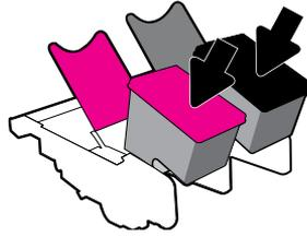
Open carriage latches and insert cartridges.
