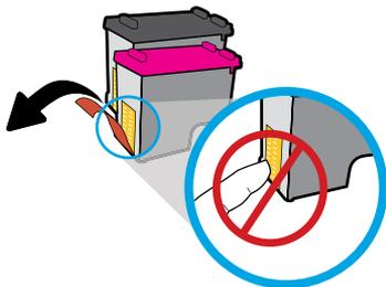
Remove plastic tape using pull tab.
