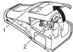
**2** Insert the rechargeable Li-ion battery into the battery compartment.
