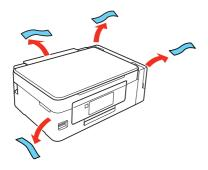
**2** Lift up the scanner unit and remove all protective materials from inside the product.
