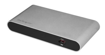
This Thunderbolt<sup>TM</sup> 3 to USB 3.1 controller adapter offers twice the performance of a traditional 4-port USB 3.1 hub, enabling you to connect a wide range of devices to your Thunderbolt 3 laptop. With dedicated USB buses, the controller adds four USB ports - two USB-A (5Gbps), one USB-C (10Gbps) and one USB-A (10Gbps).
