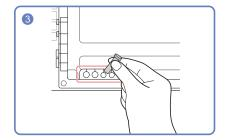
Insert and keep the removed Silicone-Bar in the marked area to ensure it is not lost.
