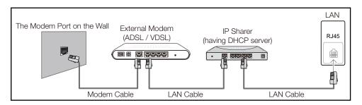
Depending on how your network is configured, you may be able to attach your product to your LAN by connecting the LAN port on the back of your product directly to a network wall outlet using a LAN cable.
