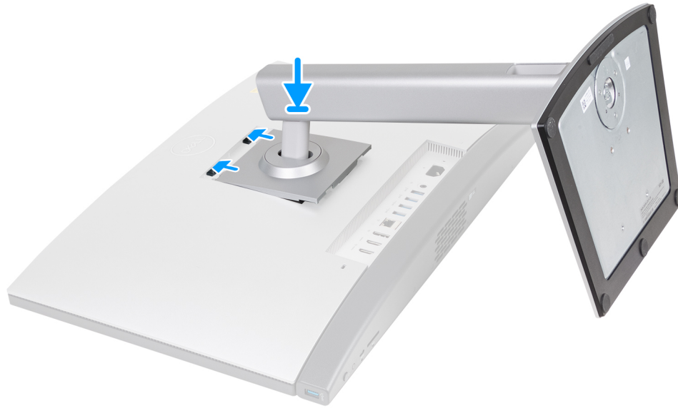
Figure 11. Installing the stand
