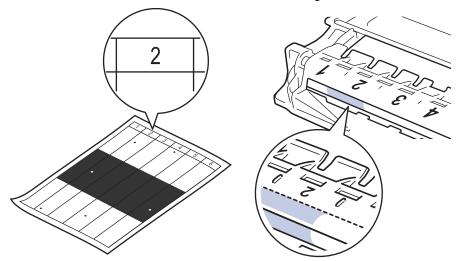
13. Turn the drum unit edge towards you while looking at the drum surface to find the mark.
