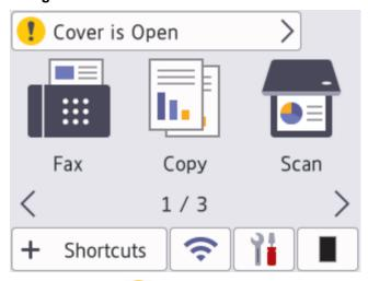
The warning icon • appears when there is an error or maintenance message; press the message area to view it, and then press to return to Ready Mode.
