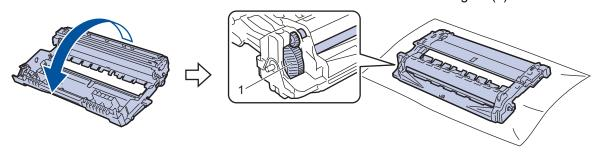
10. Use the numbered markers next to the drum roller to find the mark on the drum. For example, a dot in column 2 on the check sheet means that there is a mark in drum region "2".
