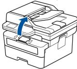
You can still use the machine while the scanner cover is up. To close the scanner cover, gently push it down with both hands.
