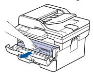
3. Clean the corona wire inside the drum unit by gently sliding the green tab from left to right and right to left several times.
