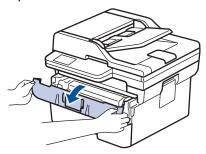
7. Remove the toner cartridge and drum unit assembly from the machine.
