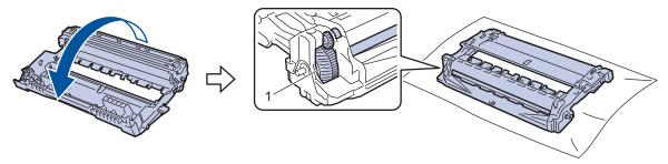
12. Use the numbered markers next to the drum roller to find the mark on the drum. For example, a dot in column 2 on the check sheet means that there is a mark in drum region "2".
