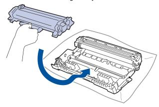
Make sure you put the toner cartridge in correctly or it may separate from the drum unit.
