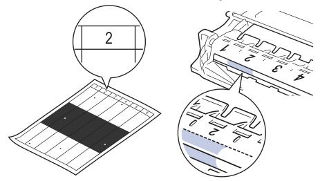
11. Turn the drum unit edge towards you while looking at the drum surface to find the mark.
