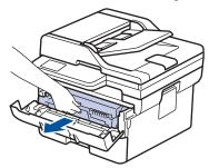
8. Push down the green lock lever and take the toner cartridge out of the drum unit.
