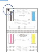
Follow the LCD instructions to print the Adjustment Sheet. The black circle mark is located in the upper left corner of the sheet.
