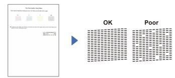
Follow the LCD instructions, and then press <code>[OK]</code>. The machine prints the Print Quality Check Sheet.
