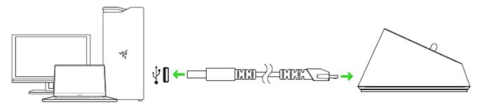
2. Insert the USB wireless dongle into your computer's USB port.
