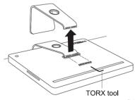
7. Align the hole in the Flange (7) with the pin on the back of your iMac, then use the Torx Tool (12) and the screws removed in the previous step to attach the Flange.
