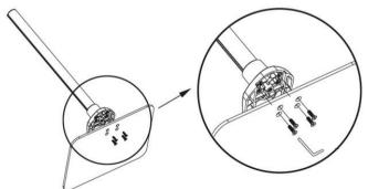
2. Attach the Rubber Feet (15) to the Base (1).
