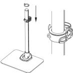
**Warning:** Ensure the Iron Position Ring is installed, and that the monitor is slid onto the Support post facing forward (over the base). The Iron Position Ring limits the ability to swivel the monitor around too far, causing the center of gravity to shift and possibly fall over
