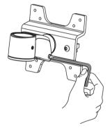
To increase / decrease swivel resistance, adjust the set screw located on the side of the Monitor Mount bracket at the Support Post, using the 3mm Allen Wrench (10).
