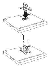
Slide the Monitor Mount (3) onto the Support Post (2) until it rests on the Iron Position Ring (5) and tighten the set screw using the M3 Allen Wrench (15).
