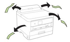
**2** Raise the printer cover and remove all protective materials from inside the product, then close the printer cover.
